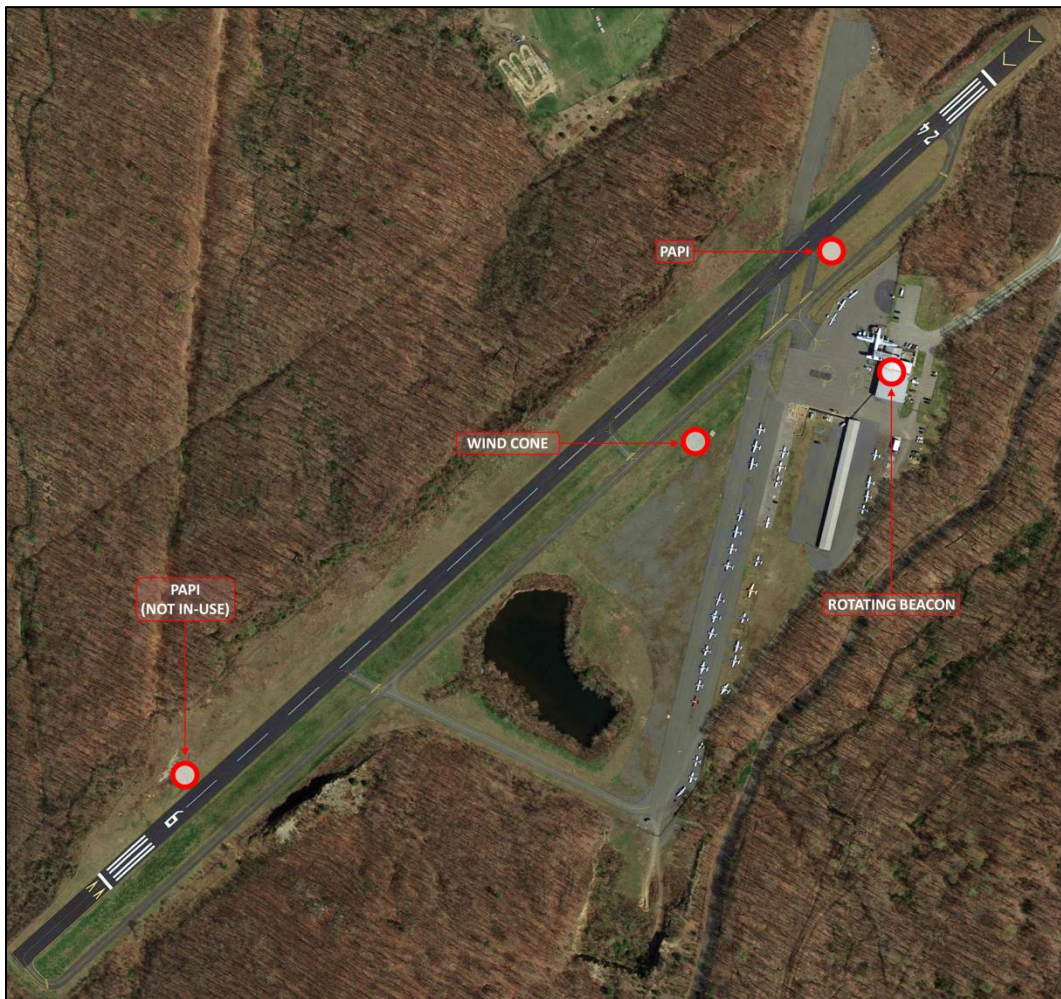
Figure 1-6. Navigational and Lighting Aids at 4N1
