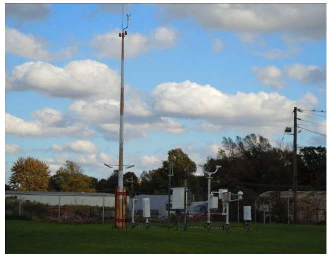
Figure 1-6: Automated Surface Observing System (ASOS)
